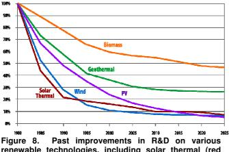
renewable technologies, including solar thermal (red curve) and photovoltaics (purple curve), have yielded impressive cost reductions.
