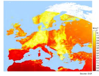
Figure 2: Solar resource assessment based on satellite data, and resulting PV electricity generation potential (PV only on roofs in settlement areas) (Scholz, 2006)
