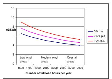
Figure 8. The costs of wind-produced power as a function of wind speed (number of full load hours) and discount rate. *Source: EWEA*
