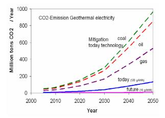
Figure 21. Mitigation potential of geothermal power plants in the world based on data of Table 6 and assumptions for emission of 120 g  $CO_2$ / kWh for today and 10 g  $CO_2$ / kWh for future technology.
