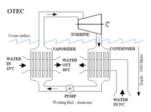
Figure 10: Diagram of a closed cycle Ocean Thermal Energy Conversion plant
