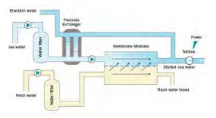
Figure 11: Diagram of pressure retarded osmosis (PSO) process using salinity gradients.
