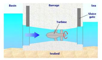
Figure 9: Tidal barrage type of tidal device.
