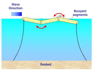
Figure 9: Pitching type of wave device
