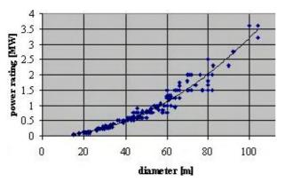
Figure 2. Rating vs diameter of wind turbine designs *Source: EWEA*
