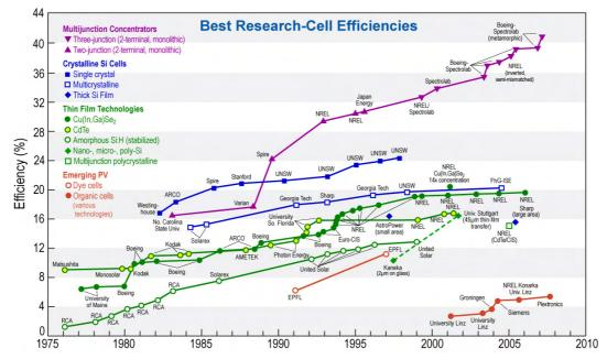
Figure 15. Improvements in conversion efficiencies for various technologies of laboratory photovoltaic cells (compiled by L.L. Kazmerski, NREL).
