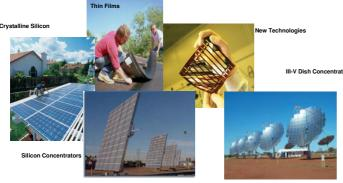
Figure 14. Various examples of photovoltaic technologies, from flat plates (crystalline silicon and thin-film devices, plus new second- and third-generation technologies) to concentrators (using silicon and III-V high-efficiency cells).
