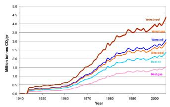
Figure 15.  $CO_2$  savings using geothermal water in Reykjavik (Iceland) compared to other energy sources 1940-2006. Total avoidance 90 million to 110 million tonnes of  $CO_2$  emissions depending on the type of fossil fuel(s) replaced by geothermal resources (Gunnlaugsson, personal communication 2008).
