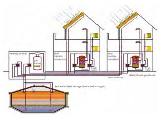
Figure 7: Scheme of a central solar heating plant with seasonal storage (Heidemann et al., 2006)
