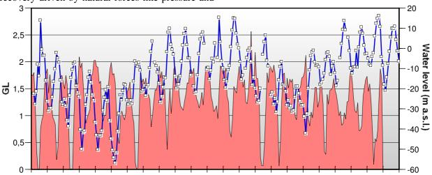
Jan 1985 Jan 1987 Jan 1989 Jan 1991 Jan 1993 Jan 1995 Jan 1997 Jan 1999 Jan 2001 Jan 2003 Jan 2007 Figure 22. Production in Gigaliters (in red) from the Reykir low-temperature field and the water level (black line with data points) in well MG-28 (observation well) from 1985 to 2007 (Ivarsson, 2007).
