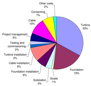
Figure 9.Estimate of capital cost breakdown for an offshore wind farm *Source: DTI. 2007a*
