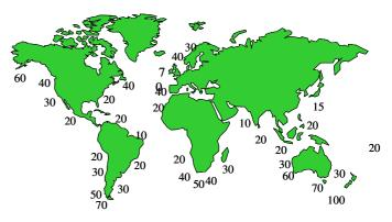
Figure 1: The highest wave activity (kW/m) is found between the latitudes of  $\sim 30^{\circ}$  and  $\sim 60^{\circ}$  on both hemispheres.
