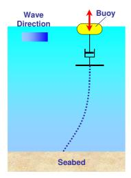
Figure 7: Buoy type of wave device.
