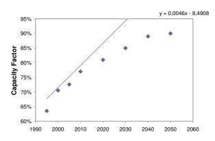
Figure 20. Capacity Factor of geothermal power plants in the world 1995-2005 and forecasts for 2010-2050
