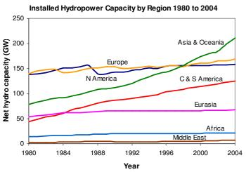
Figure 3: Growth in hydropower capacity by region (EIA, 2007)
