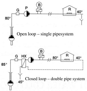
**Figure 10. Two main types of district heating systems.** G=gas separator, P=pump, B=boiler, R=radiation heating, HX=heat exchanger (Dickson and Fanelli, 2003).
