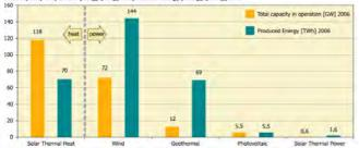
Figure 7. Estimated global capacities, energy outputs, and 2005 and projected costs out to 2030 for solar thermal energy [IEA 2007].
