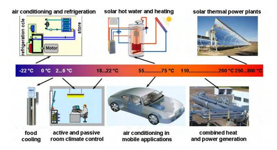
Figure 8: Examples and temperature range for thermal storage (Müller-Steinhagen et al., 2007)
