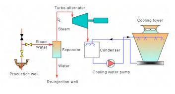
Figure 7. A schematic diagram of a geothermal condensing power plant
