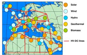
Figure 6: Concept of a HVDC based trans-continental ,super grid' (Trieb et al., 2007)
