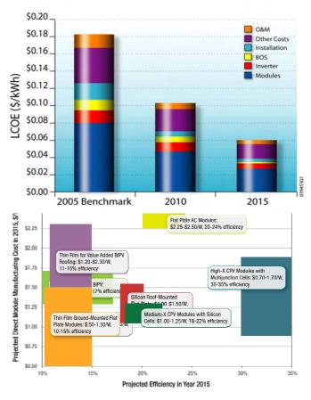
Figure 13. The roadmap to PV electricity in parity with conventional grid power includes scaling up manufacturing, improving processes, designing products driven by applications, and developing products for easy installation.
