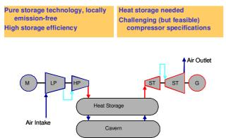
Figure 4: Adiabatic compressed air energy storage system
