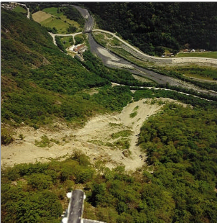
Figure 8.3 Closer view of the shallow movements shown in the previous figure. The irregular morphology of the slope reflects however deeper deformation in the rock massif
