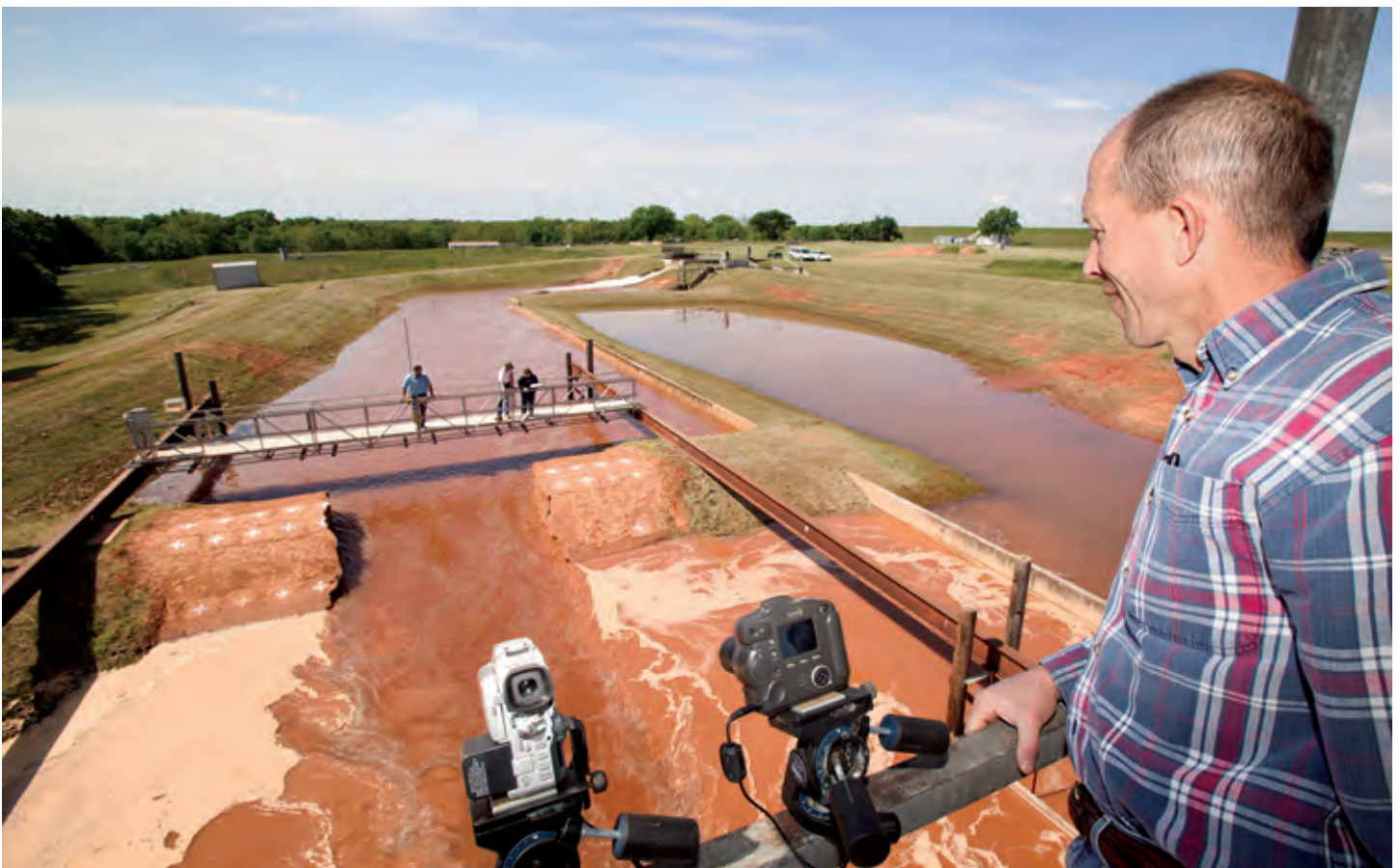
From an observation platform overlooking a test dam, hydraulic engineer Greg Hanson records the test for use in computer modeling. Photo courtesy of USDA, ARS, Stephen Ausmus.
