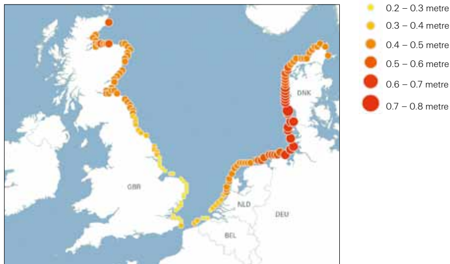
Projected increase in surge height for peak events (IPCC scenario A2, including 37cm sea level rise).
