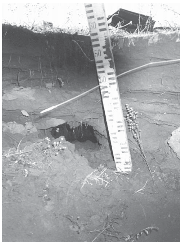
Figure 2. Cavity where ice wedges have melted out. Experimental plot 4, Maya (Photograph by P.V. Efremov).
