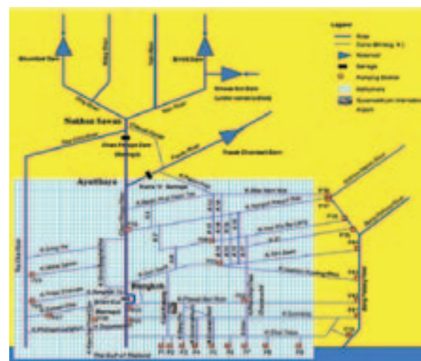
FIGURE 2.1 ■ Hydrometeorological Model Schematic for Chao Phraya Watershed
