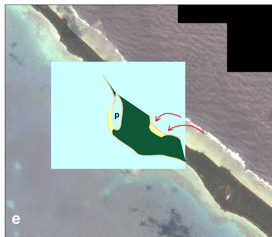
(e) With sand supply blocked the channel on the ocean side quickly in-filled (red arrows). On the lagoon side the unstable sandy spit moves and changes shape since the supply of sand from the ocean has stopped. Low areas which were once part of the lagoon / channel are isolated from the sea and over time become freshwater ponds (p).
