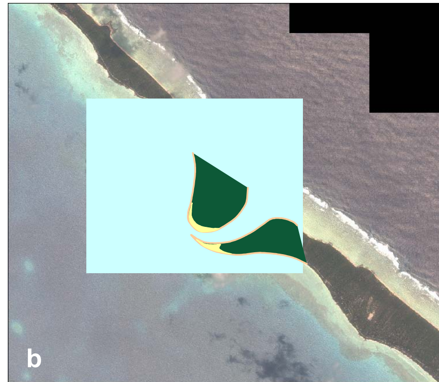
(b) Over time the channel fills with sand and eventually becomes narrower and shallower. The persistent northern sand transport pattern not only supplies this sand from the ocean reef through the passage but on the lagoon side it pushes a sand spit extending to the north.
