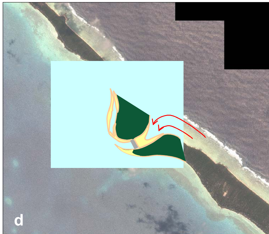
(d) At some time, about 70 to 100 years ago, villagers built a causeway across this channel (this area is still known as “ Terawabono ” – “the blocked channel”). This stopped the supply of sand moving to the lagoon side.
