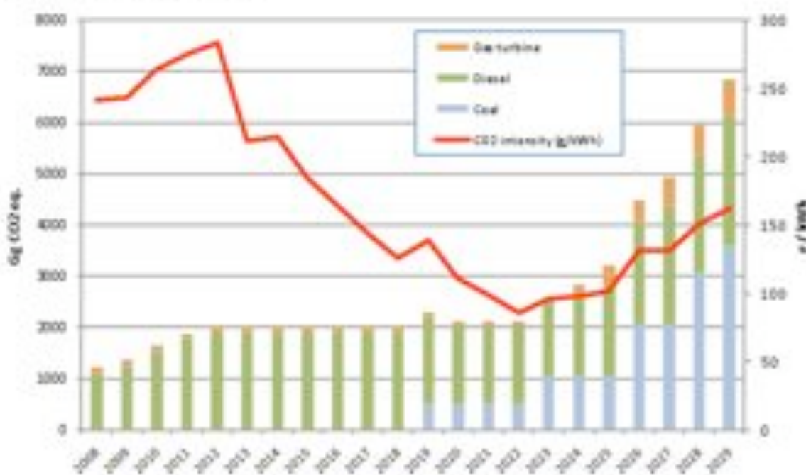
Figure 26. Projected CO 2 emissions by generation type (2008-2029) 17 , and CO 2 intensity of generation (g/kWh) 18
