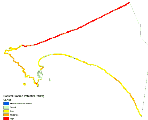
Figure 13: Coastal Erosion Potential Layer for Dakar, Senegal Aggregated to 250m Cells.
